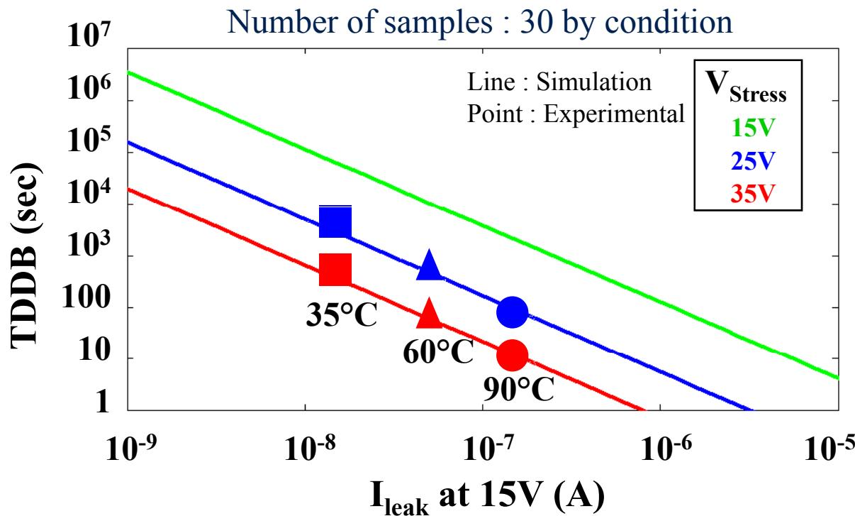
$$\text{TDDB} = A \times (I_{\text{leak}} \text{ at } 15V)^{-p}$$
