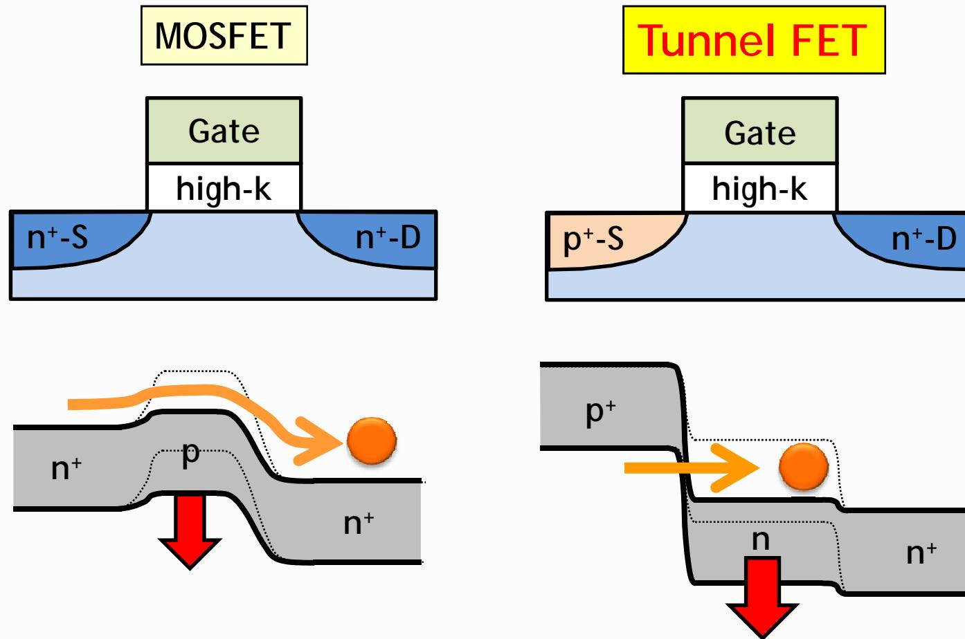
Carrier flow is determined by thermal-injection mechanism
