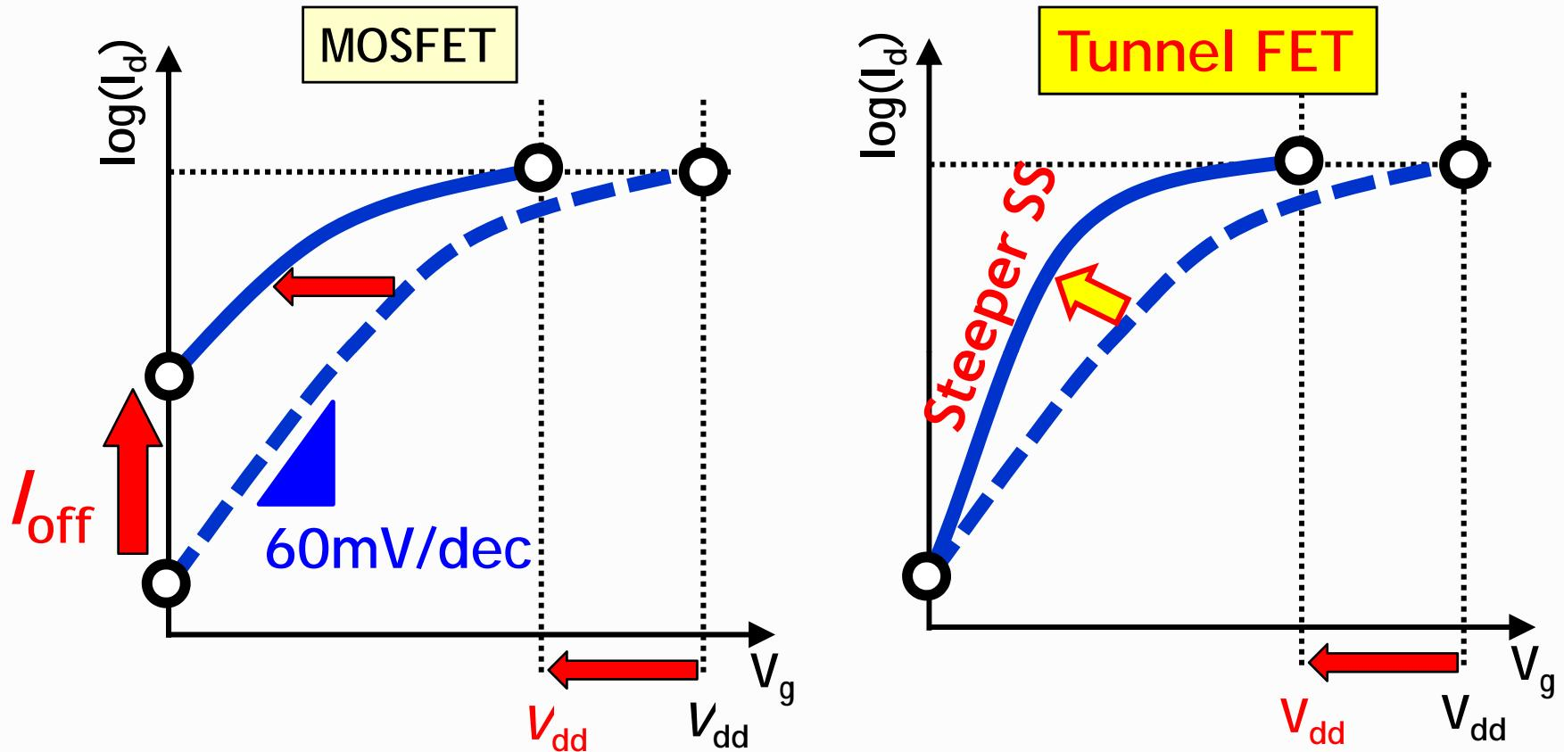
Conventionally  $V_{dd}$  scaling causes a significant increase in  $I_{off}$  due to the lower limit of SS ( $\sim 60\text{mV/dec.}$ )
