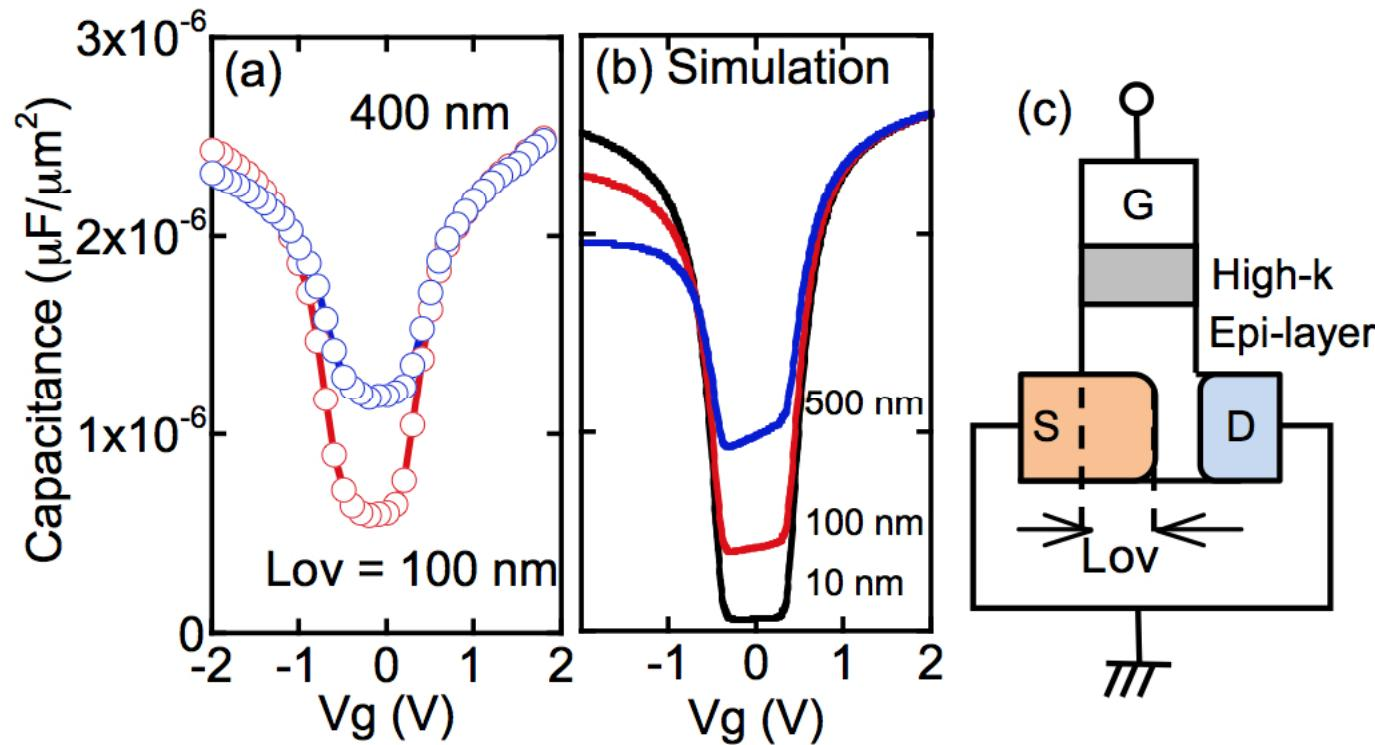
Fig. 4 Typical CV characteristics for the PP-capacitor of VTM TFETs. Variations in the different  $L_{OV}$  are shown. (a) Experimental and (b) simulation results. (c) Measurement setup.
