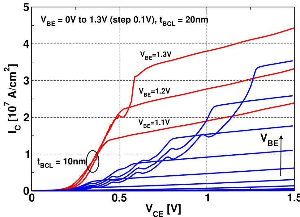
Even if BCL barrier is low or absent,  $V_{CE}$  still affects  $I_c$  through the electrostatic influence on  $Q_{GR}$  and  $V_{Dirac}$ .
